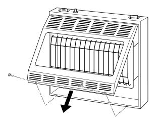
Figure 7 - Removing Front Panel Of Heater
